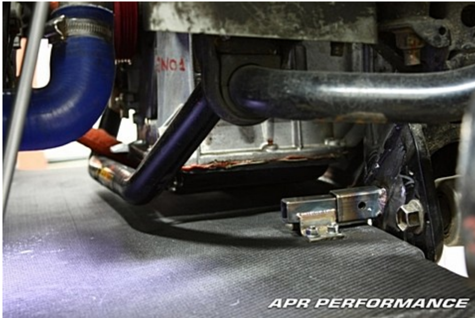
Example: Custom support bracket connects to steel bumper beam on a Mazda Miata ( http://slickauto.net/ )
