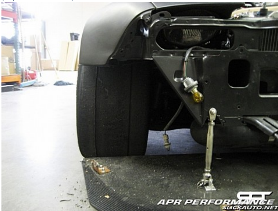
Example: Custom support bracket connects to subframe on a Nissan 350z
