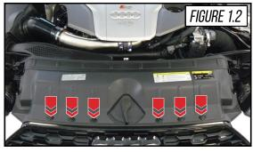
Remove the upper radiator cover by lifting up at the arrows in **Figure 1.3**. Lift and slide forward to remove the cover completely.
