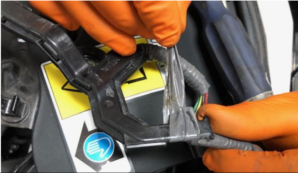
9. Remove the tape around the wiring harness. We now need to remove the plastic cover.
