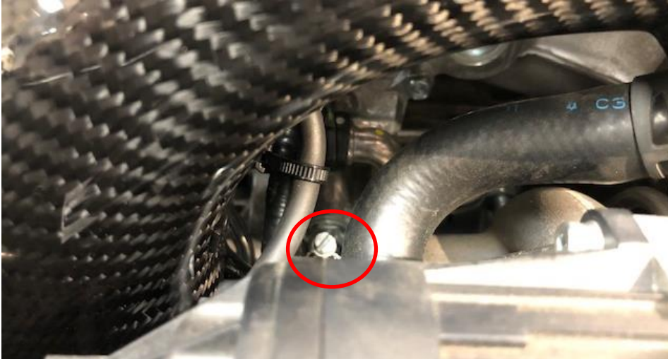
33. Secure the remaining hose clamp around the silicon coupler at the turbo side. Do NOT OVERTIGHTEN. This just needs to be hand tight.
