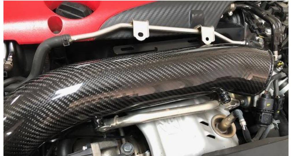
26. Carefully lower the tube into place.
