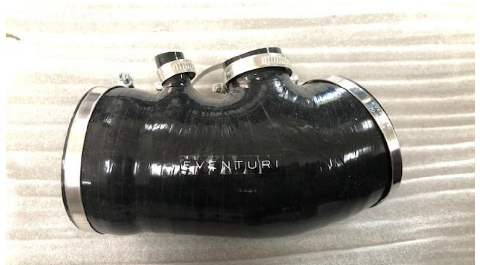
34. Take the new Silicon hose and use the 2 small hose clamps and the breather boss from your previous silicon hose removed from the intake (removed in step 2).
