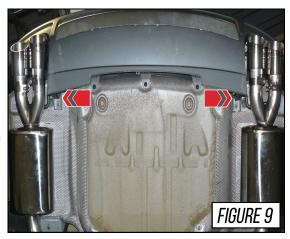
Tighten all the supplied Accu-Seal clamps to 40 ft/lbs. Once the system is fully tightened, go back and adjust the tips if necessary.
