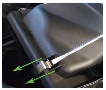
Pop the factory air box lid clips open and remove the lid. Bend and remove the factory clips from the side of the airbox by bending them outwards down almost horizontal. Then bring them straight up and push down to remove. They will need to change shape a little before they can be removed. The silver heat shield will need to be temporarily removed for this step.
