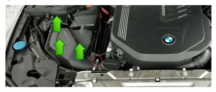
There will be a round rubber grommet and a rectangle rubber grommet stick to the airbox bottom. These must be removed and put back on the car before reinstalling the factory airbox bottom.
