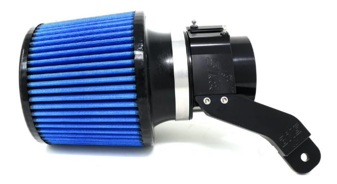
Attach the "MAF" temperature sensor with the provided 7/64" allen screws to the BMS intake.
