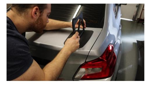
**2.10.** With the trunk opened, thread the nuts onto the studs using the 10mm socket, and tighten to about 6 ftlbs.
