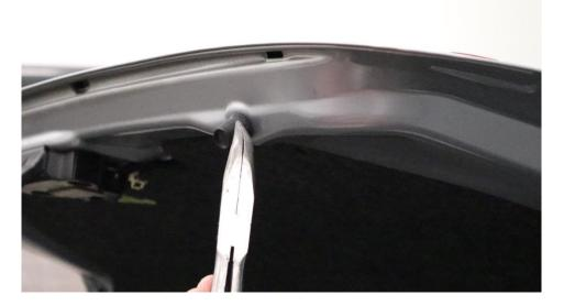
**2.15.2.** Once the bumper is removed, you will be left with a hole that you will step out to 3/8" with your step drill bit.
