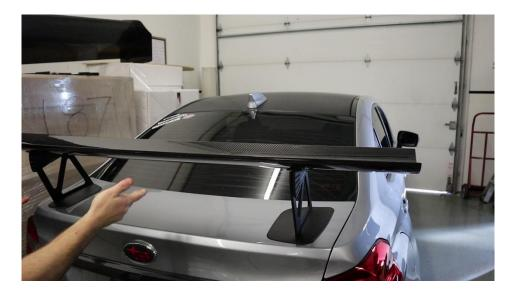
**2.13.** Grab (4) M6 BHCS, (8) M6 washers, and (4) M6 nyloc nuts. Install the front bolts first, using a 3mm allen wrench and a 10mm socket. Tighten to 6 ftlbs.
