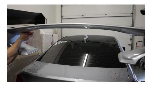
**2.6.** With the spoiler removed, it should reveal a dirty foot print where dirt and grime will tend to collect over time. We recommend cleaning this area at the very least, however you may want to polish this area with a buffer to make sure the paint looks the same as the rest of the trunk. The base plates for the wing uprights do not cover the exact footprint of the factory spoiler.
