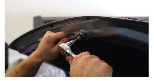
**2.16.** Grab the low profile SHCS and jam nut, and adjust the jam nut so that it matches the height of the factory bumper.
