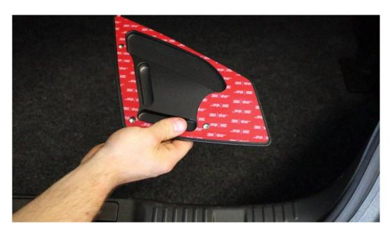
**2.7.** Locate the two 40mm long studs, and install them into the trunk mount by using a 3mm allen wrench to bottom the stud so that it is snug.
