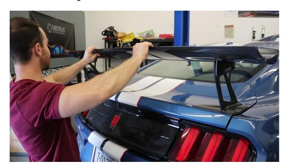
2.17. For AOA, below is a guideline of what we have designed and tested internally. Every install and car can vary from this slightly. To ensure proper AOA, you should lay a straight edge from front to rear of the wing and check the degree measurement \*in relation to the ground plane\*. The center holes are designed to be at 0, 5, 10, and 15 degrees.
