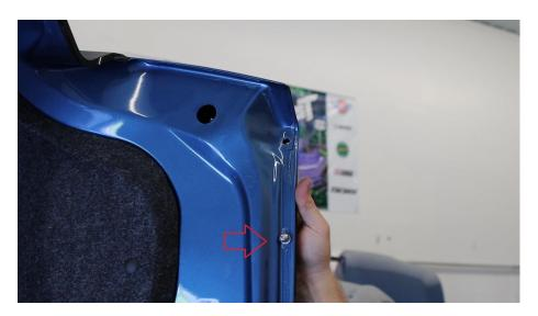
**2.10.** Once the mount is stuck to the trunk, remove the previously installed 16mm long BHCS, and re-install the OEM strengthening plate with two 16mm long BHCS with a washer. Torque the bolts to 6ftlbs.
