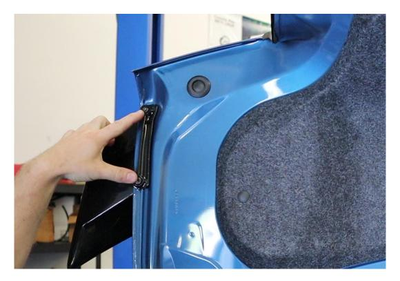
**2.3.** Next, we will remove the rubber plug exposing a 10mm nut and spacer. Remove the nut, and spacer being careful not to drop them into the inner trunk skin. If the spacer is still stuck on the trunk after removing the nut, you may want to put the trunk lid down and tap on it to try and "knock it out".
