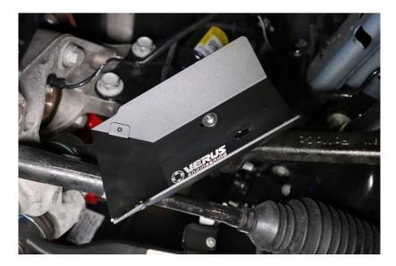
**2.5.** Next, install the bottom bolt using 1x 25mm BHCS, 1x washer, and 1x nyloc nut. This time you will not use a washer on the back of the control arm. Refer to the picture below. Again, do not tighten yet.
