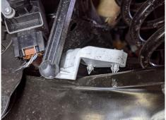
3. Disconnect the electronic damping control wires from the damper (Figs. D.9 - D.11).
