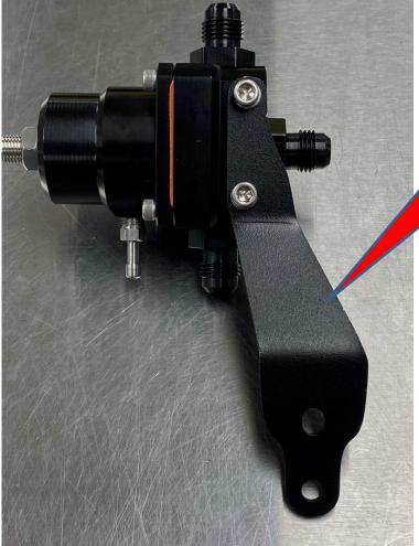
Install the FPR Bracket using the hardware supplied with the Aeromotive FPR. Pay attention to the orientation of the bracket in all 3 photos.
