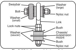
Fig.3 Whiteline eye/pin type link.
