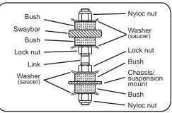
Fig.1. Whiteline double pin type link.
