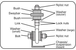
Fig.2. Whiteline pin/eye type link.
