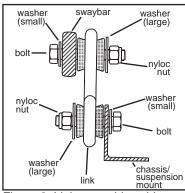
Figure 2. Link assembly guide.
