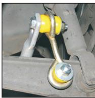
Photo 3. Link assembly - front view.
