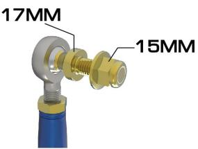
7R Repeat for the passenger side. Clocking and positioning will be a mirror image of the left. Reinstall wheels and torque lug bolts to 103 ft lbs.
