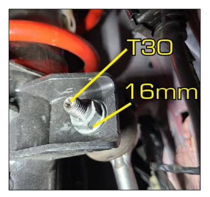
4F Unbolt the end link from the sway bar using a T30 socket and 16mm as well. Remove the factory end link from the car. Mark "left" on the end link for reference.
