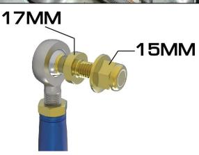
7F You should now have the end links installed with only the right-hand jam nut loose to clock the rod end angle.
