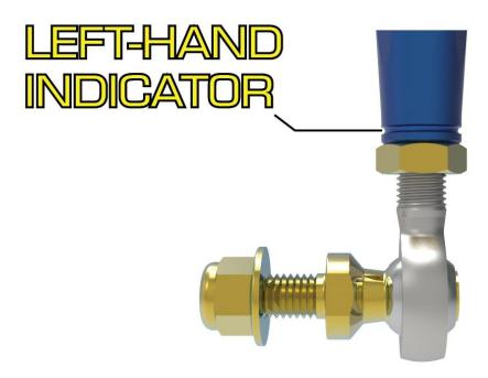
6F Install the end link in the same manner as stock removal. Install the left-hand (tightened) end on the strut and right-hand end on the sway bar end
