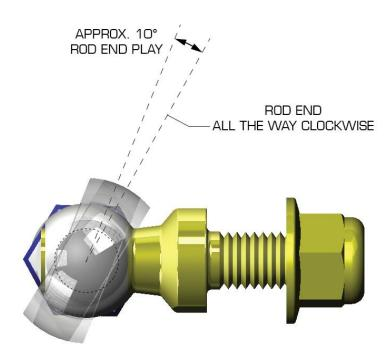
Next, turn the wheel all the way to the right and make sure the end link has the same amount of rod end play. This will ensure your rod ends will never run out of articulation when steering.
