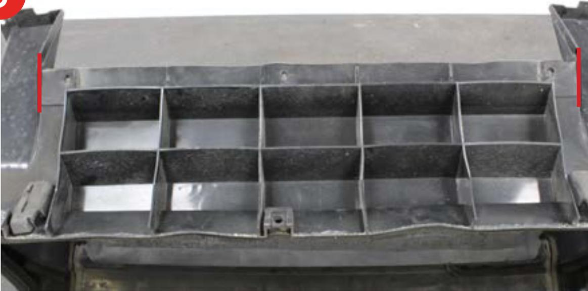
6. Install the supplied side plates and factory lower lip support brackets. Use the supplied hardware to install the side plates. The side plate lower profile will push and form the lower part of the air duct downwards. Trim more if needed as down in step # 6 to get the plate and profile correct.
