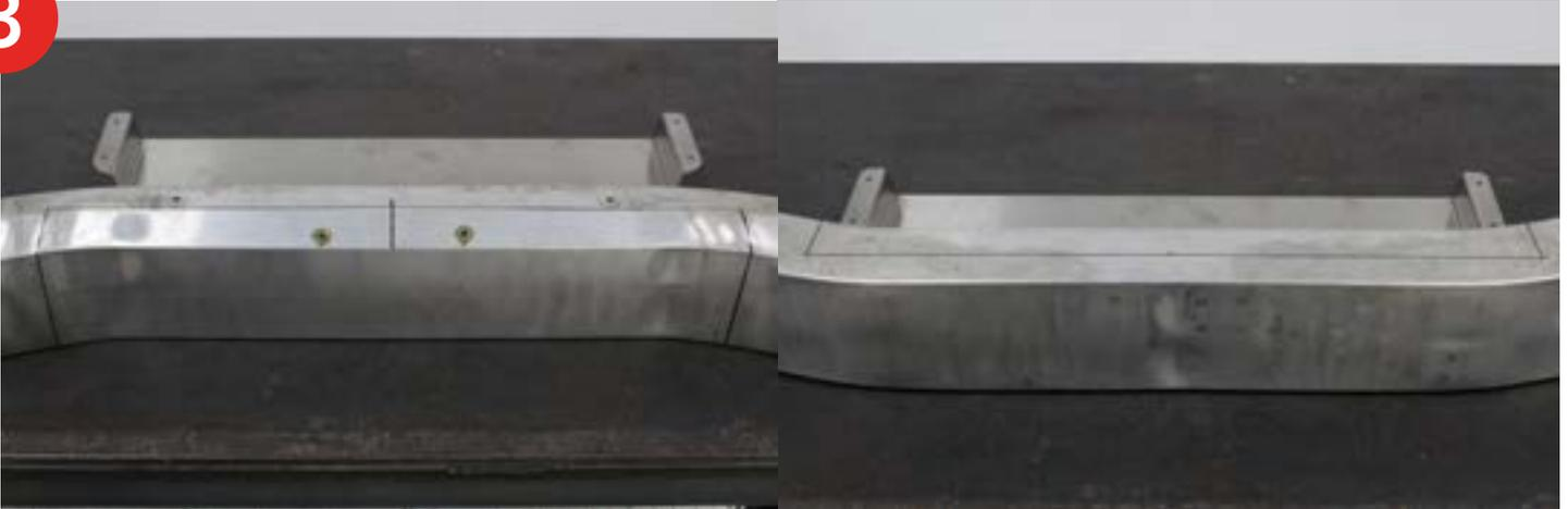
4. Set the crash beam in front of the intercooler installed on the vehicle to make sure your marks are correct.
