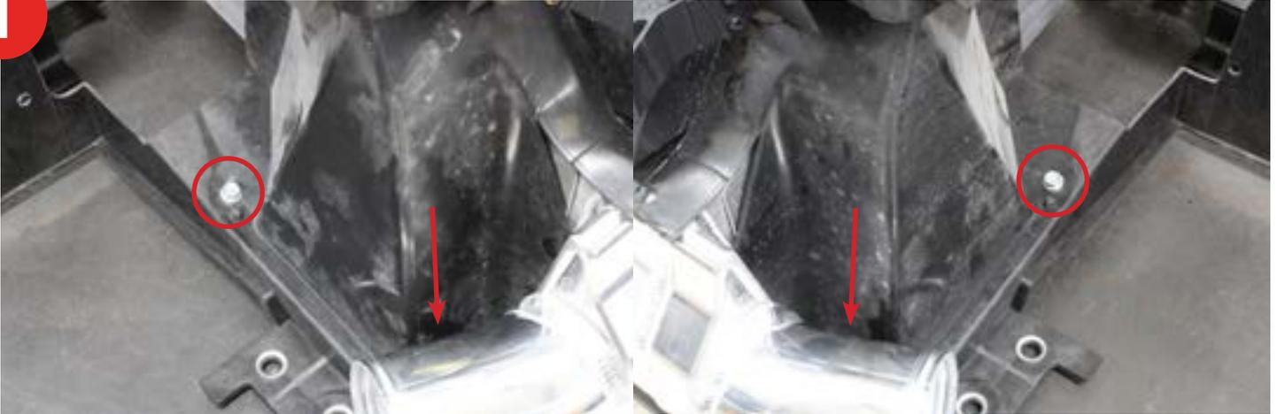
2. Reinstall the core support and intercooler assembly back onto the car. It can be permanently installed. Make sure to lift the intercooler support as high as it will go before tightening. The weight of the intercooler will pull down on everything slightly. If this is not done, the bumper and hood alignment will be off.
