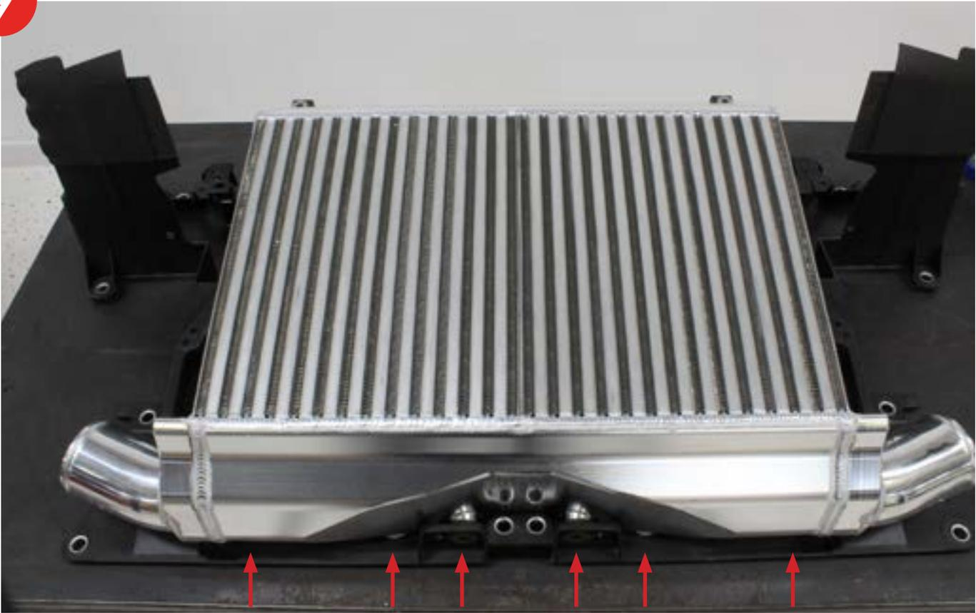
10. In the hardware kit locate the two red support brackets. Install the brackets with the supplied M6 and M10 hardware. Leave loose for the moment as final adjustments will be made when installed on the car. Make sure the bracket with the small square cut hole is installed the right side / passenger side of the car. This hole is for the outside air temp sensor.
