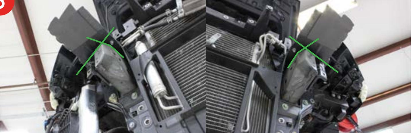
6. Remove the support and highlight the marked area shown using your traces. This area needs to be cut out. The after pictures are also shown below.
