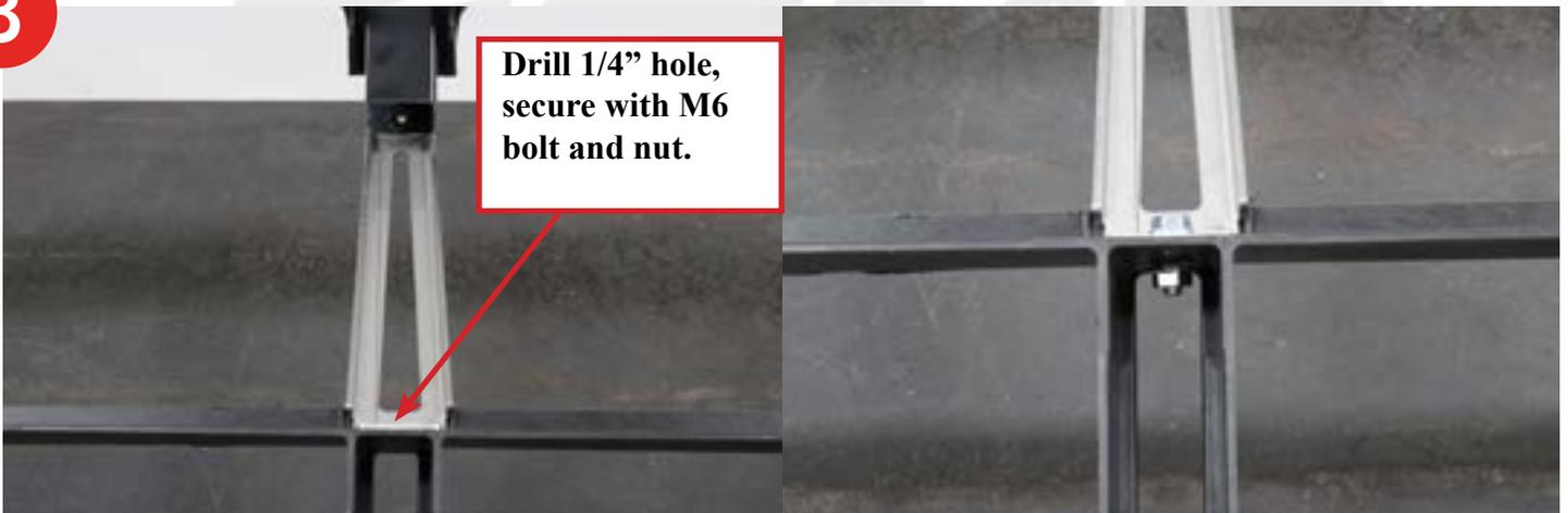
Make sure the bracket hole aligns with the threaded hole in the support. Trim as necessary.
