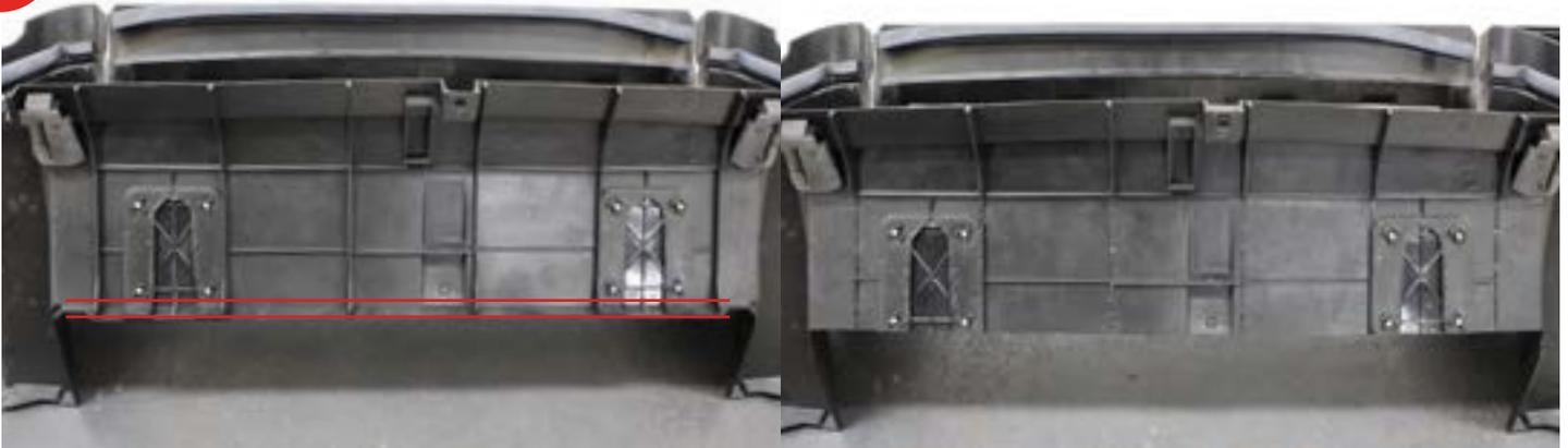
6. Next cut 2 slits in the lower part of the duct. No material will be removed in this step. The slits allow the duct to flex to a new profile. Only cut the area shown, do not over cut this area. Trimming in a later step may be needed.
