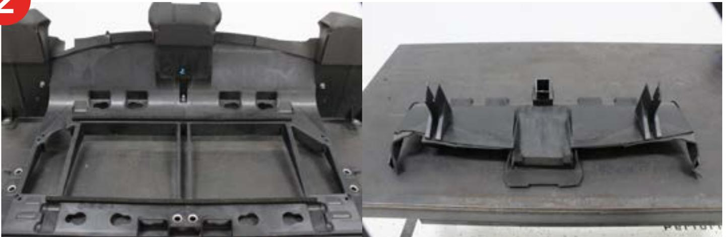
3. See the areas noted in red in the next few pictures, these will be the cut lines. We found the best way to cut the support is with a large tooth air saw at low speed. The low speed will keep the material from melting back together when cutting and will leave cleaner lines. There will also be one area you will need to cut through a metal support.
