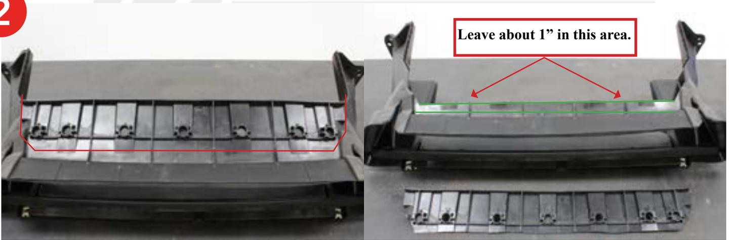
3. Cut and remove the lower mounts. Make sure to cut them off as flush as possible to the air duct.
