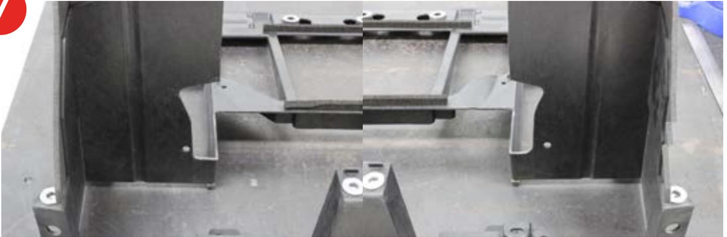
8. In the hardware kit, locate the stainless steel support bracket. Install the bracket as shown and mark the lower hole shown on the support. Drill a 1/4" hole here for attaching the bracket. Use a supplied M6 bolt and nut to secure the bracket. Make sure the upper hole of the bracket aligns with the support's threaded hole. Adjust and trim as necessary.
