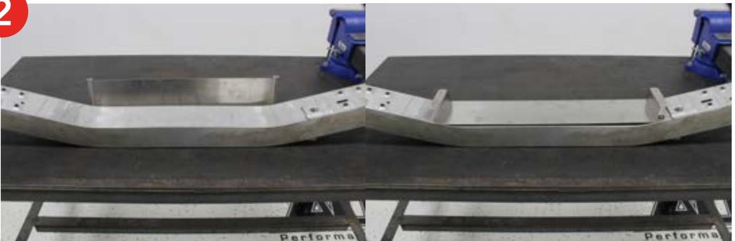
3. Set the panel on the top and bottom of the beam and mark it. Use a straight edge to draw the final lines.
