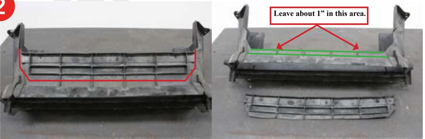
3. Remove the webbing as shown in the pictures below. The webbing needs to be removed so the duct will flex around the bottom the intercooler.
