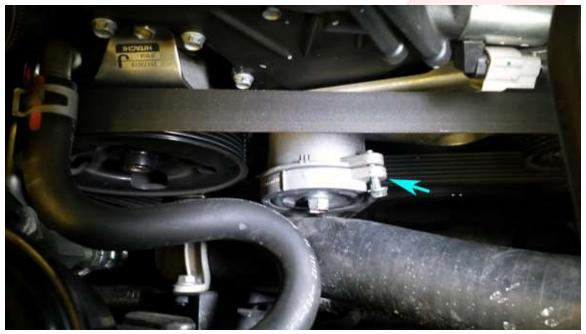
2. Use a 14mm socket/ratchet combo to remove 2 serpentine idler pulleys on
