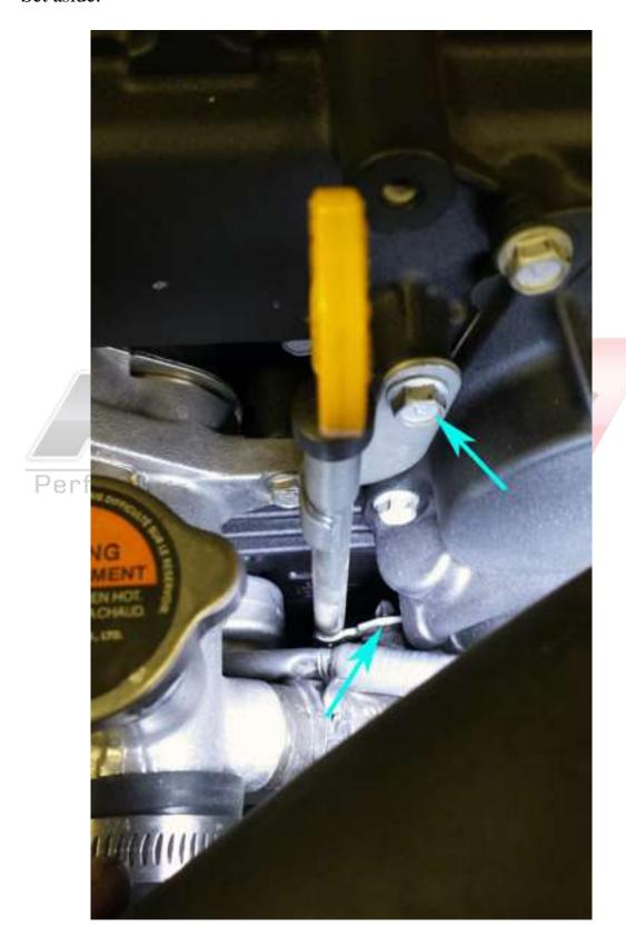
4. Slide new Alpha dipstick tube into place on engine This step will go smoother if a dab of grease is used on the o-ring. Re-attach cam solenoid wiring at this time.
