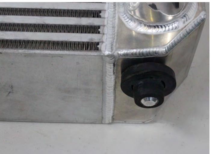
**13.** Install the AMS intercooler. The new AMS Intercooler is much larger and heavier than the OEM unit, so a second set of hands here is recommended. Reinstall the lower intercooler support plate using the OEM hardware.
