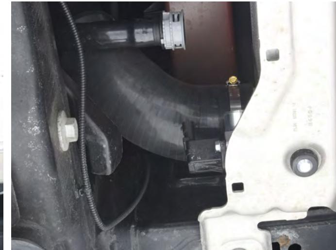
**16.** Remove the grey clip from the bypass valve recirculation tube. Release the tabs by turning the gray retainer in the direction you did to remove it. Slide it off the tube. Clean the surface on the end of the tube.
