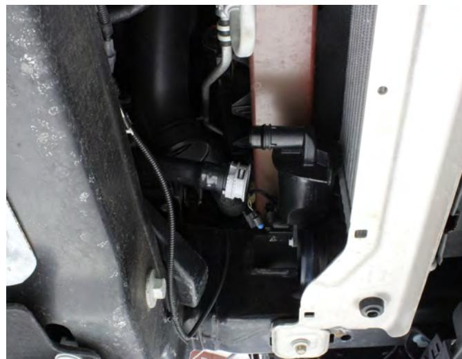
**06.** Unbolt the lower intercooler mount from both sides of the frame. Carefully lower the intercooler down to gain access to the bypass valve wiring harness. This harness may be a little tricky to remove. The harness is held in place by two fir tree style clips into the top of the intercooler. Release these clips and remove the intercooler. Below is a picture of the harness and intercooler removed from the truck to give you an idea of what is going on.
