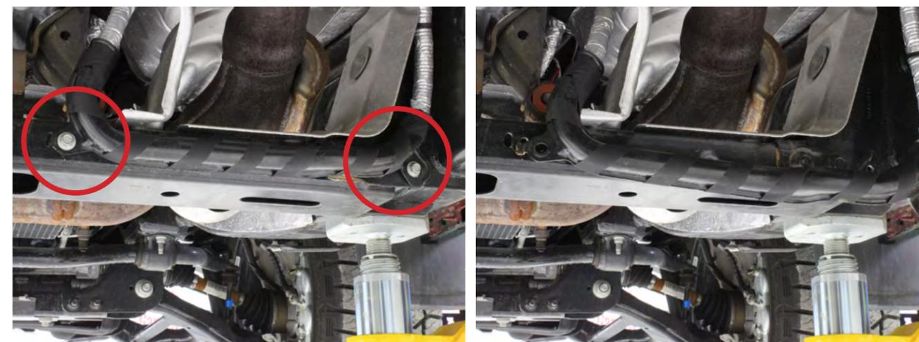
04. Remove the heat shield on the top of the transmission cross member that bolts to the frame.
