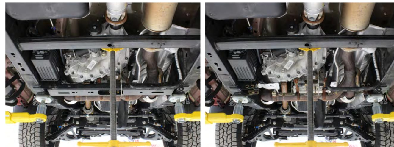
08. Remove the exhaust hanger top clamp and transmission mount bolts on the driver's side.
