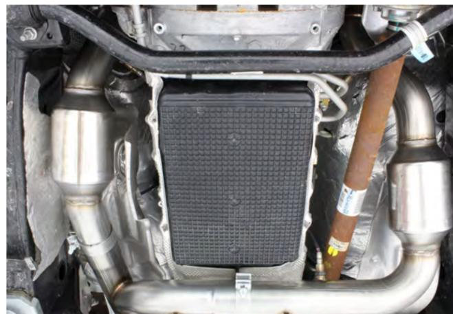
20. Reinstall the O2 sensors. The passenger rear sensor will not route through the heat shield as it did with the OEM downpipe. It will now route over the top of the heat shield and around. This was the reason for releasing all the clips on the rear O2 sensor harness in step #17.
