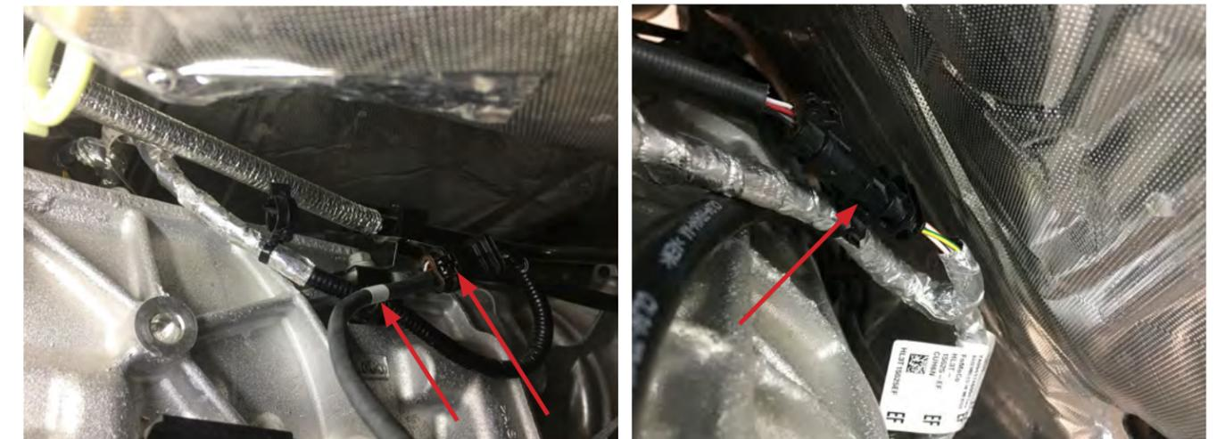
18. Loosely assemble the AMS downpipe and install it in the truck. If the OEM downpipe was cut to remove, the AMS downpipe will need to be slipped together in the truck piece by piece. Leave the two-bolt connections and clamps loose at this time.
