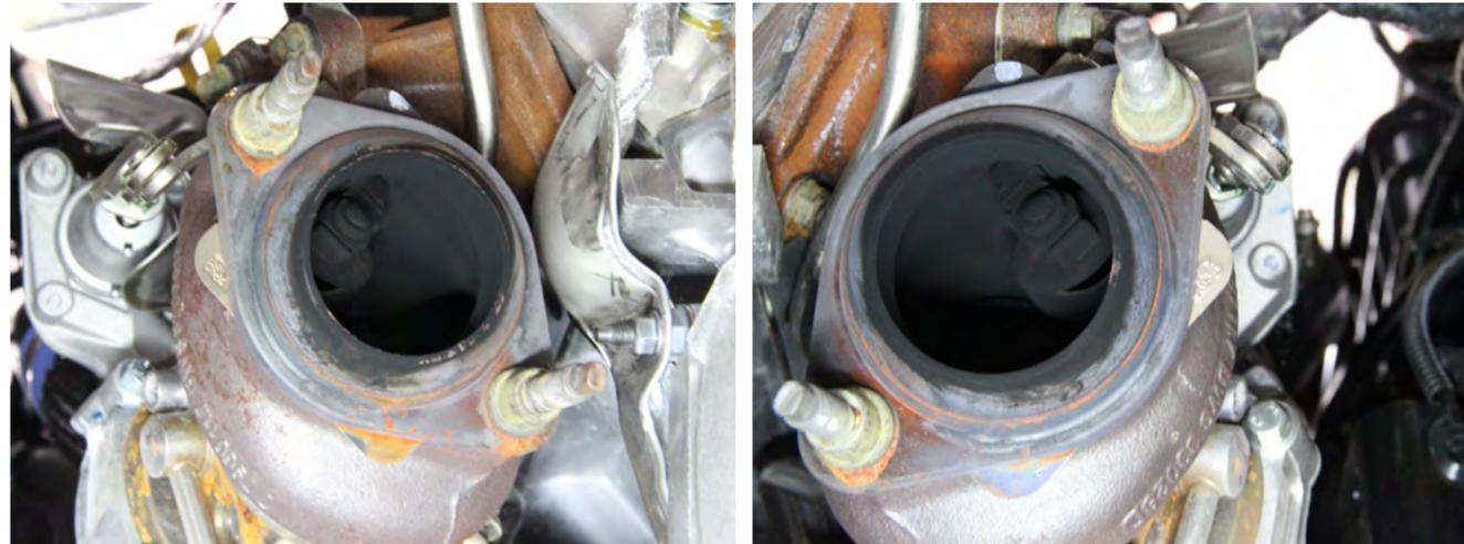
15. Use a 10mm or 3/8" stud extractor to remove the stud from the turbine housing outlet flanges. This may take a little heat on the turbine housing to get these studs to move.
