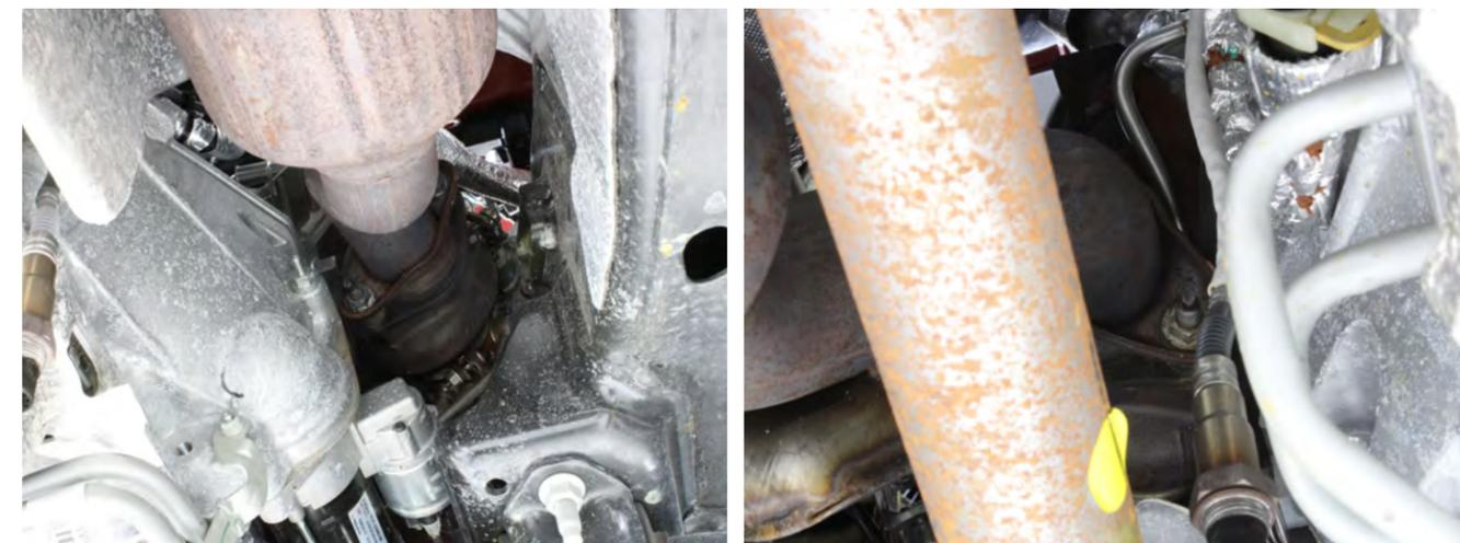
13. Push the exhaust over to the right-side frame rail and hold it there using a strap. Pull the harness disconnected from the transmission cross member in step #3 towards the rear of the truck. You will need to slip the downpipe down and around the harness. Carefully remove the OEM downpipe assembly. It will take a little back and forth to work it out.
