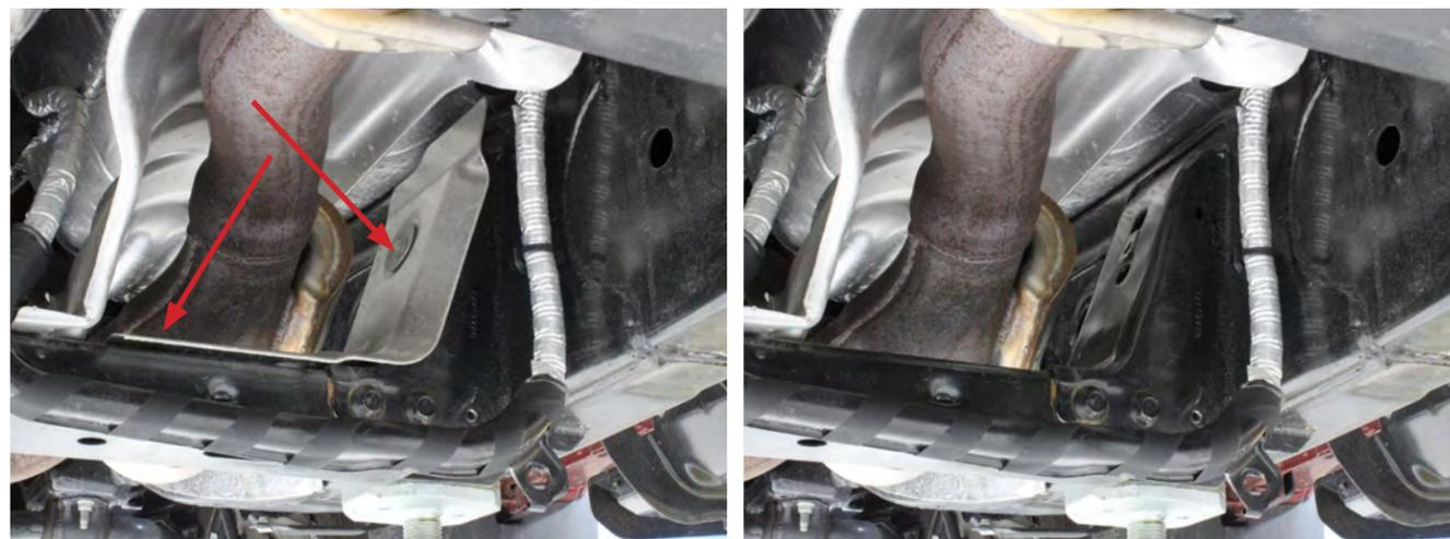
05. Remove the two bolts holding the heat shields on the top of the transmission cross member. There is one on each side of the transmission. These heat shields do not need to be removed, only the bolts.
