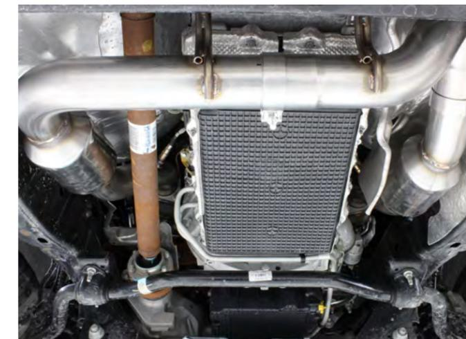
19. Reinstall the transmission mount and cross member. Once everything is installed and the downpipe is aligned, tighten the two-bolt flanges first starting with the connection at the turbo. You must be careful to tighten these flanges evenly. Failure to do so may result in exhaust leaks and/or damage to the ball seal and flange. Next tighten the two-bolt flange to exhaust, followed by the band clamps.
