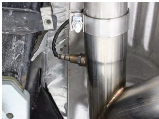
21. Make sure tie up any loose harnesses away from heat sources and rotating drivetrain parts.
