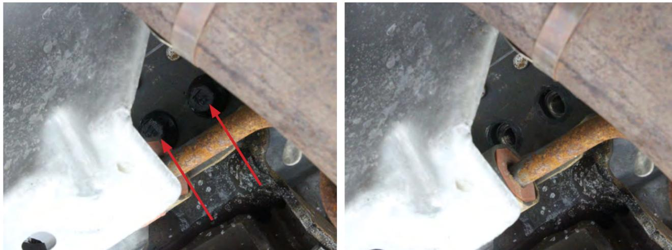
10. Remove the transmission mount from the vehicle.
