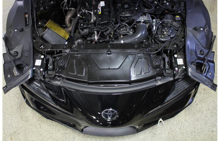
2. Remove the front hood seal and the six 10mm bolts underneath. Gently pull the nose piece of the bumper free of its mounting clips. With that out of the way, you can gain access to the 13mm cover panel bolts. Loosen the four front bolts and remove the rest. Unclip the hood release cable and the panel will slide backwards and then pull up.
