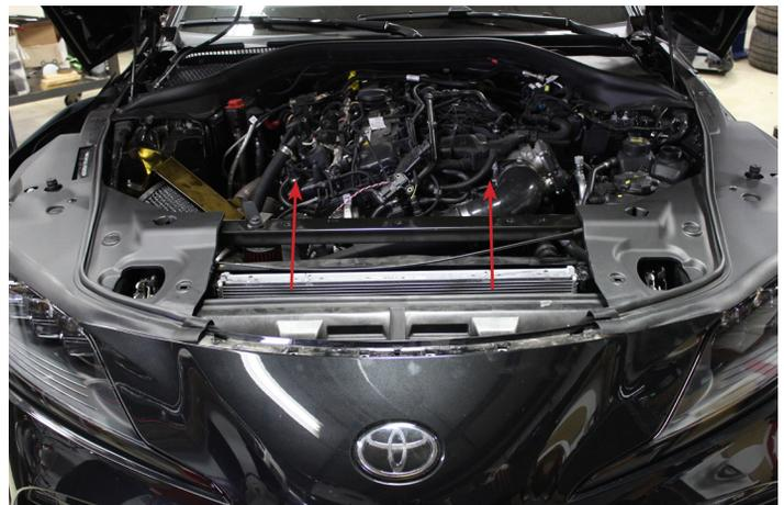
6. With the factory heat exchanger removed, the mounting brackets for the transmission cooler will need to be slightly modified to account for the extra width of the AMS heat exchanger. There are a few different ways to do this, explained in the following steps.
