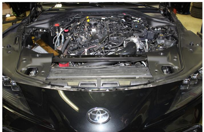
3. Next, remove the two T30 screws holding the plastic radiator cover in place. It is clipped into the fan shroud and will need to be unclipped to remove. If the cover is difficult to remove, try lifting up on the fan shroud slightly to create more clearance for the cover.
