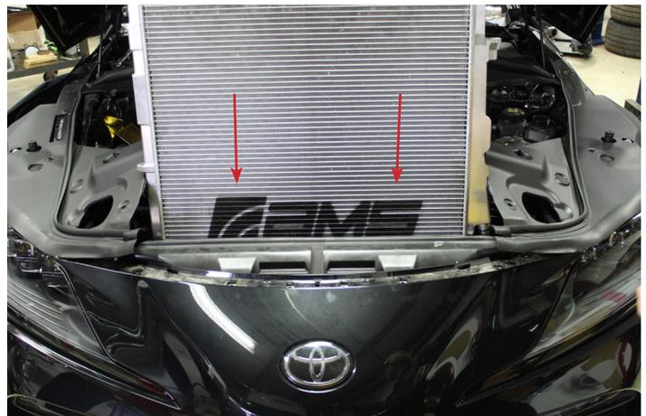
9. Once the AMS heat exchanger has been fitted, the rest of the installation is a reverse of the disassembly process. Make sure the heat exchanger fittings are properly clipped in place before installing any cover panels or refilling the system. All covers and hardware are installed back in their original locations.
