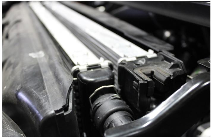
5. With both fittings removed, the factory heat exchanger can be lifted out.
