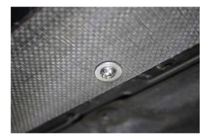
**2.18.** To complete the install, we must install a sheet metal screw and washer into the chassis in the frontmost location. Do so by using a T35 Torx Bit.
