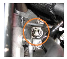
**2.12.** We now want to remove the PCV check valve from the piece shown in 2.10. Also shown below.
