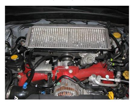
**2.3.** For this install, we have to remove the intercooler if you still have a TMIC (Top Mount Intercooler). Start by removing the (2) 10mm bolts that hold the vent tube on circled below in red.
