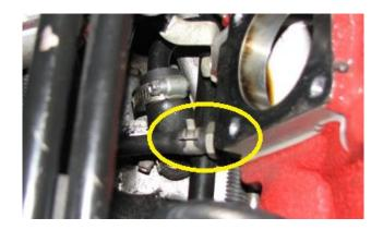
**2.9.** Now we can remove the PCV system that is near the turbo, circled in blue below.
