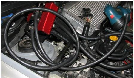
**3.5.** Install the shorter hose onto the overflow as shown below. Try to spill as little coolant as possible by using a clamp.
