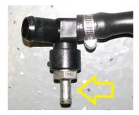
**2.13.** Install this in the open location on the AOS as shown below. We recommend using Teflon tape or Teflon sealant.
