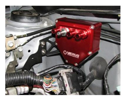
**2.19.** Install the OEM bracket removed in 2.16 and install this on the bolt locations located on the left of the bracket. Use the M6x1.0 x 16mm BHCS, fender washers, and serrated nuts to install this.
