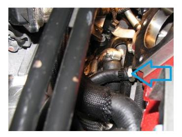
**2.23.** Finish off the hose routing by installing the two vent hoses as shown below. Routing is your choice but this is how we routed ours. The hoses are highlighted with yellow lines below.
