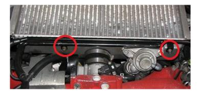
2.4. Remove the BPV by taking the two 12mm bolts off, shown circled below in yellow.
