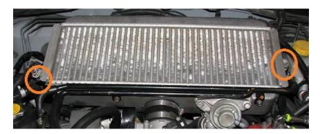
**2.7.** Remove the charge cooler from the car.
