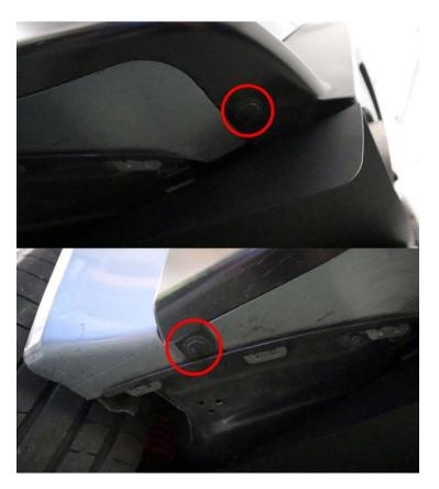
**2.4.** Once the plastic rivets are removed, pull the tab out of the way in the frontmost location as shown below. Note, if you ever plan to replace the black factory bumper trim, that is shown in the photos, you will want to remove the trim in the rearmost location as well. We do not plan to replace this piece, so we did not remove it for ease of install.
