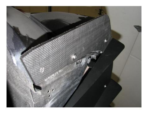
**2.11.** Mark the third and final location by using a Sharpie and then remove the loosely installed rear spat. After the rear spat is removed, you should see something like the image below
