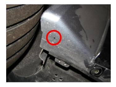
**2.12.** Now we need to drill this location and install the final rivet nut.
