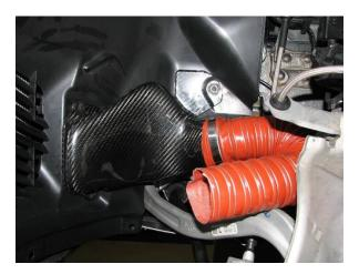
2.17. Once the hose is installed and tucked away, it is time to install the backing plate using the OEM hardware. Torque spec for these bolts is 6 ft/lbs. Note the orientation of the backing plate below as there are left-hand and right-hand sides. Again, this is the driver side of the vehicle on a left-hand drive model.
