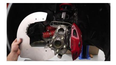
2.18. The backing plate should be installed as shown below.
