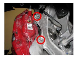
2.7. Remove the rotor by removing the 6mm Allen head bolt from the rotor as shown below.
