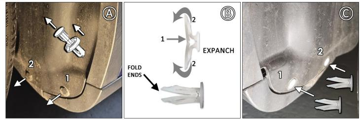
**FIGURES D** Place mud flap logo-side facing rear of vehicle against lower mounting points. Install SCREW .5BLKSS and WASHER SMWASH through mounting points 1, 2. Do not fully tighten.
