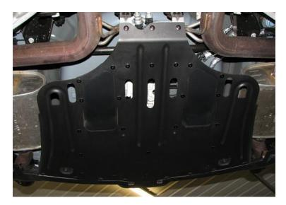
**2.4.** We begin by removing the push clip rivets in the rear (red circles) and the (2) 10mm bolts (yellow circles). The (2) push in clips that are circled in blue will stay for now.
