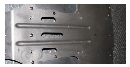
**2.16.** Using the BHCS, washers, and nylocs, we can install the inner strakes. Note that there is a left and right hand side. The front two tabs face outward, while the rear two tabs face inward as shown below. We use a washer on both sides for these strakes.
