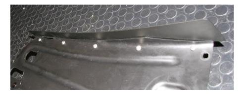
**2.12.** With the correct outer strake, washers and nylocs, we can install the strake as shown below. When fully tightening, ensure that the strake's rear tab lines up with the cutout as shown in step 2.8. Tightening torque should be 6 ft-lbs.
