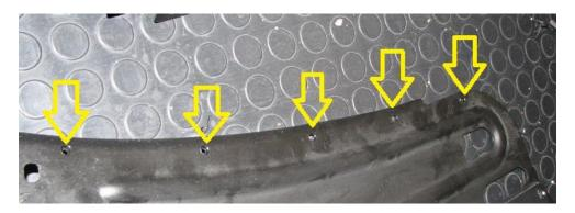
**2.10.** Flipping the diffuser over, we can debur these holes with a debur tool of your choice.
