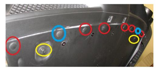
**2.5.** Moving to the front of the diffuser, we can remove the two 10mm bolts that hold the front on and let the diffuser rest on the hook clips.
