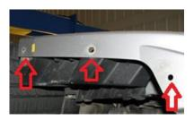
**2.5.** We want to make sure that we are installing the rivet nuts into the black plastic and not through the bumper as well. This is shown below.
