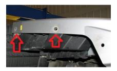
2.4. We will be installing rivet nuts in these three locations shown below. \*Note: If you have our rear diffuser installed, this has already been done.\*
