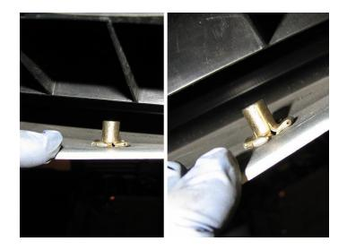
**2.9.** From the bottom, bolt the rear spat onto the car with the supplied bolts.
