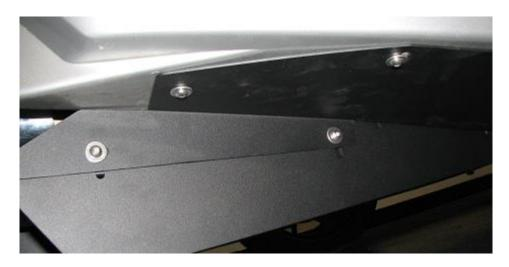
**2.19.** Serrated nuts will be used on the back (inside) side of these (4) points per side.
