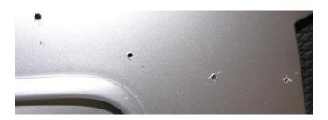
**2.13.** Using the countersink, clean the holes from any burrs from drilling.
