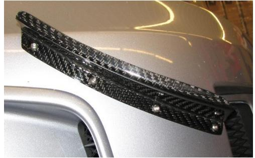
**2.15.** Reaching your hand behind the front bumper you can start threading on the washer and then the nyloc nut.
