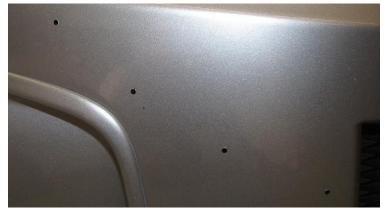
**2.12.** Increasing the drill size to 11/64" and open the holes to 11/64".
