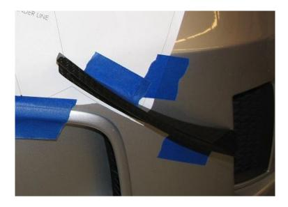
2.10. Mark the center of the holes with a center punch or tap. You will use the paper templates for the top (2) holes but will need to use the dive plane for the most forward hole.
