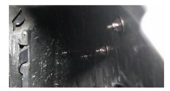
**2.16.** Tighten torque should be no more than 40-60 in-lbs. The nyloc will resist backing off, so the fasteners only need to be snug to the bumper.
