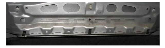
**2.7.** We can now install the hood scoop block-off. The (3) tabs on the top of the block-off go between the plastic hood scoop piece and the hood (yellow arrows). The (3) holes on the bottom of the plate bolt to the push-clips we installed in 2.6.
