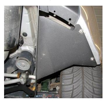
**2.13.** Finally, we move to the rear brackets. Install the rear brackets as shown below in the hole that had a plastic rivet in previously.
