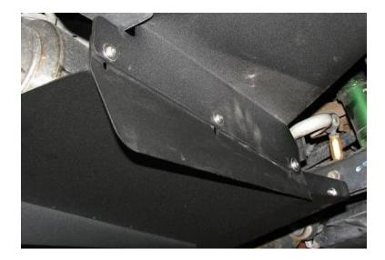
**2.24.** Once all bolts and nuts are installed, tighten all button head cap screws to approximately 10 ft-lbs. The serrated nuts, when tightened, will resist backing off.
