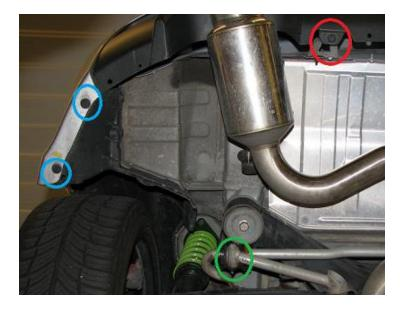
**2.5.** Starting with the front mounting points, we install the bracket under the sway bar mount utilizing the factory supplied hardware; which should be a 12mm hex bolt. Leave this loose for the meantime.
