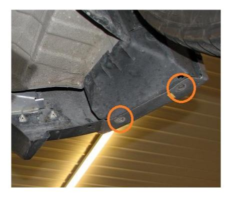
**2.8.** We will be installing the plastic rivet nuts on the front most hole, this is shown below.
