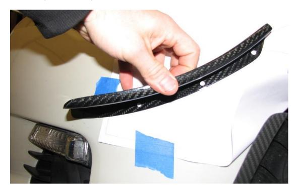
2.8. Mark the center of the holes with a center punch or tap. You can use the paper templates for the top (3) holes but need to use the dive plane for the most forward hole.
