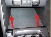
Remove the screws securing the center console.
