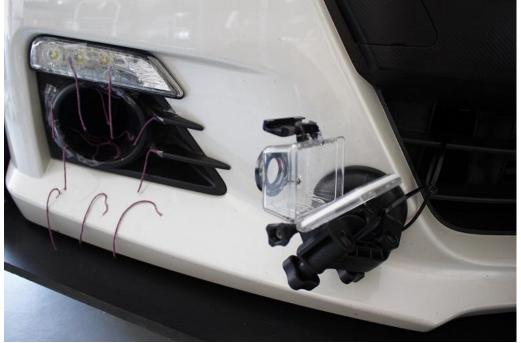
Figure 3.1: Test Setup for Tuft Testing
