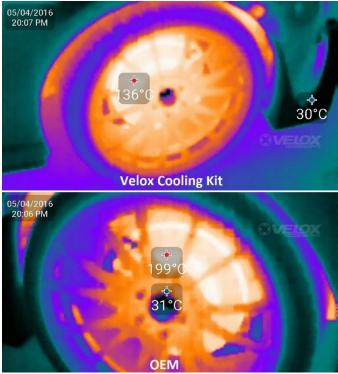
Figure 5.5: Hot readings directly after power braking at 75 MPH for 1 mile
