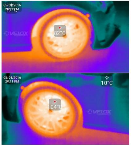
Figure 5.6: Temperature taken after 2.0 miles driving at 75 MPH with minimal brake use
