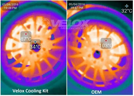
Figure 5.3: Cold readings directly after driving one mile at 40MPH with minimal brake use
