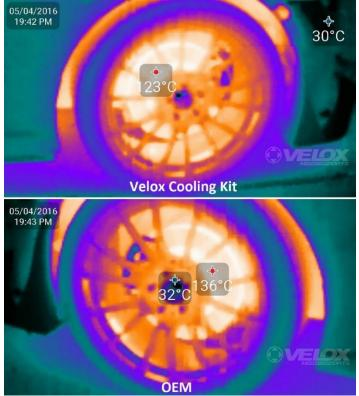
Figure 5.2: Hot readings directly after power braking for a mile
