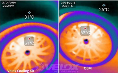
Figure 5.4: Control 2 showing rotors have leveled out in temperature after 12 minutes
