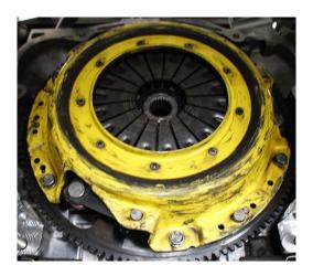
**2.7.** Install the Verus Engineering cover while using the OEM hardware. Ensure that the ground wire (circled in green) remains under the 12mm bolt and the bolt still goes through the ground wire.
