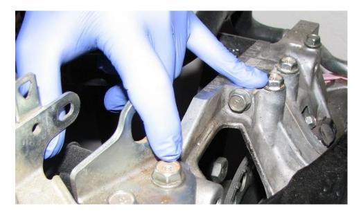
**2.5.** On car, this is where the bolts are located. The bolt circled in red is a 14mm. The bolt circled in blue is a 12mm.
