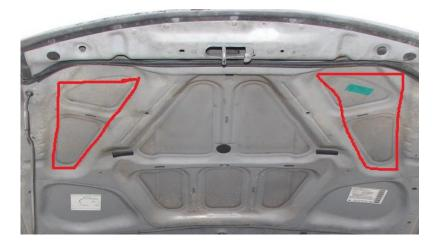
**2.6.** We will start by laying down a piece of painter's tape on the left and right sides. From the corner of the hood, we measure up 7.5" as shown below and lay a piece of tape down.
