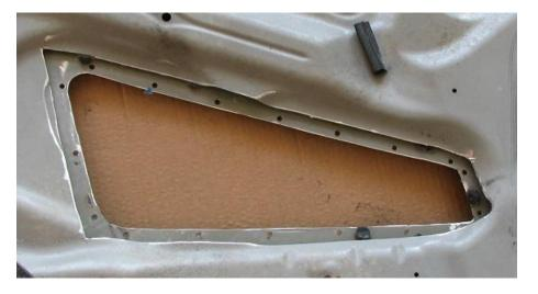
**2.21.** Again, repeat the same steps on the other half of the hood. The picture below shows the structural pieces removed from the hood.
