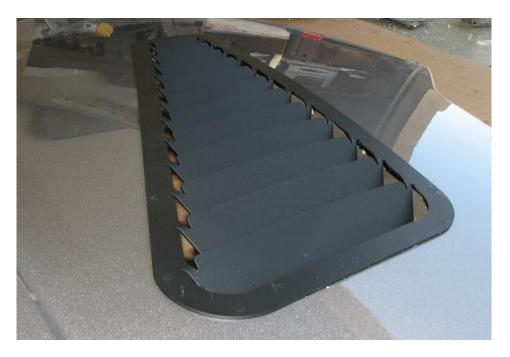
**2.27.** The wickers are installed from the bottom side of the hood louver. These increase evacuation of under hood pressure and temperature. However, some do not find them aesthetically pleasing which is why we make them optional.
