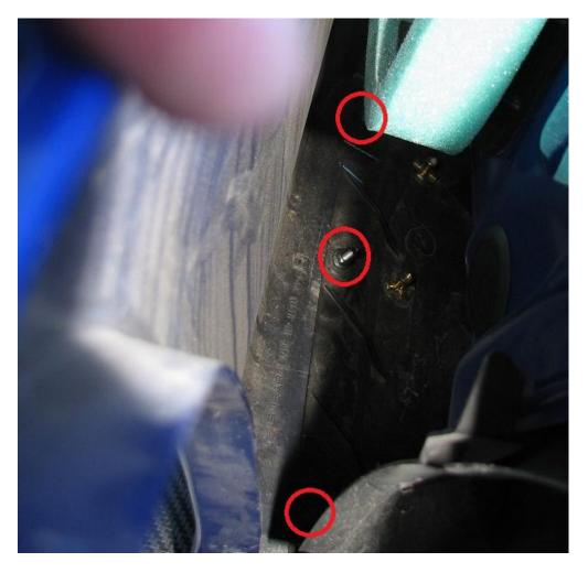
**2.5.** With access to the top of the underbody plastic obtained; we can remove the (3) plastic rivets on the bottom side of the bumper where the rear spat will be installed.
