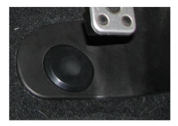
**2.14.** Install the supplied pedal stop by twisting it on the OEM stud. This will take a bit of effort at first, then the threads will form within the material and thread on easier.
