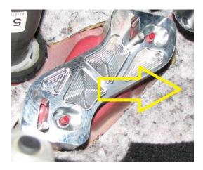
**2.11.** With the spacer torqued down, we can install the throttle pedal on the two bolts. You can adjust the throttle pedal vertically up and down. **We suggest starting with the throttle pedal tightened down in the middle of the spacer.**
