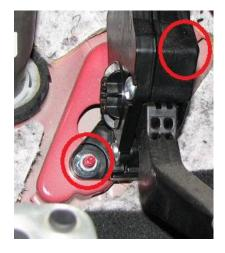
**2.6.** Unplug the throttle pedal electrical connection which is on the top of the pedal and move the throttle pedal to a safe place.
