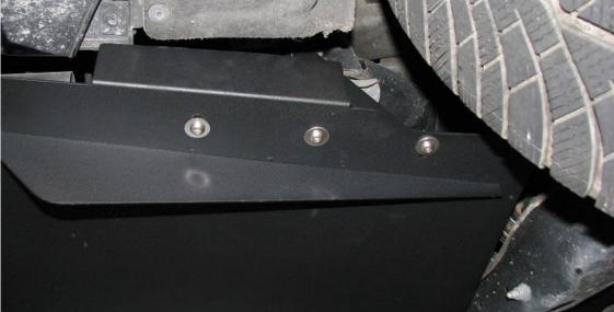
**2.19.** With the car on the ground and no rake, the diffuser strakes should be level. If the car does have some rake, you need to match the underbody's angle with the level of the bottom of the strake. Shown below is a car with no rake.
