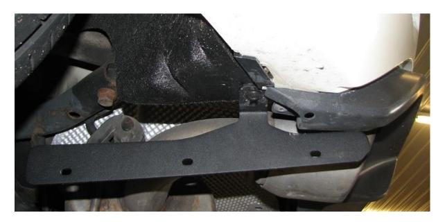
**2.9.** Finally, we move to the rear brackets. Install the rear brackets as shown below in the unused hole.
