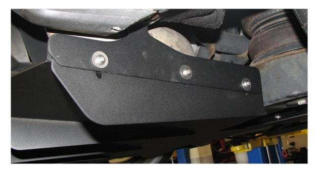
**2.18.** Once all bolts and nuts are installed, tighten all button head cap screws to approximately 10 ft-lbs. The serrated nuts, when tightened, will resist backing off.
