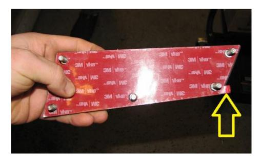
**2.16.** Using the supplied washers and nuts, install the mount onto the trunk. Tighten the nuts to roughly 6 ft-lbs. They are nyloc nuts and will resist backing off.
