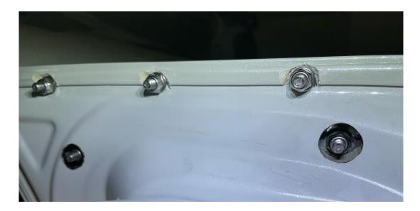
**2.17.** Using the supplied M6 x 1.0 x 16mm Long Button Head Cap Screws and a washer, install the uprights onto the trunk mounts as shown below. Tighten to roughly 6 ft-lbs.
