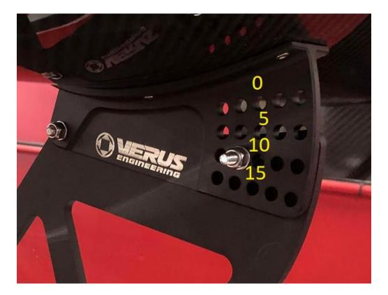
**2.21.** To finish installing the rear wing, we have to install the endplates. We offer both carbon (upgrade) and sheet aluminum (standard). Both install the same. We include aluminum washers for M4 FHCS, and O-rings to reduce marring of the aluminum of carbon fiber. Install the O-ring on the washer, and install into the endplate and rear wing as shown below. Snug the bolts, they are M4 and do not need much torque.
