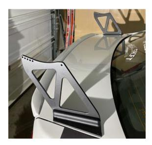
2.18. The rear wing is now ready to be installed. Use the M6 x 1.0 x 25mm long button head cap screw, washers, and nyloc nut to install the rear wing onto the uprights. Note that the wing mount is on the \*outside\* of the upright.
