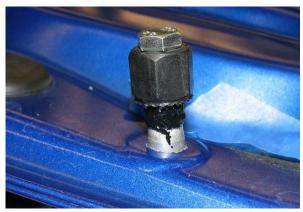
**2.27.** With the rivet nut installed into the trunk, we can install the M6 socket head cap screw with jam nut.
