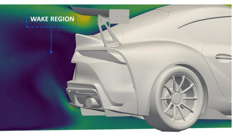
The Velocity Plot shown above is used to visualize the wake region behind the car. The blue zone behind the vehicle is the wake and minimizing this as much as possible will reduce drag.
