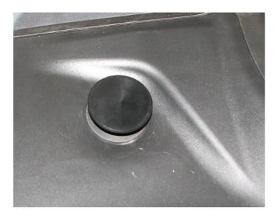
**2.28.** While slowly closing the trunk, watch the stop and see how close it comes to touching the trunk plastic. You will want the stop to hit this location when fully closed to reduce the amount of movement on the trunk at speed. This will take a bit of trial and error.
