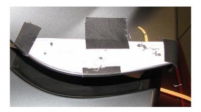
**2.8.** We need to open this hole to 1/4" for the studs to slip through. Depending on how accurately the holes are drilled, the holes may need to be slightly enlarged to slide the stud through the trunk.
