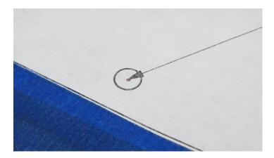
**2.7.** Using a 1/8" drill bit to start, create a starter hole for all of the holes. Drill as perpendicular (90 degrees) to the surface as possible. Keep in mind, the trunk is plastic.
