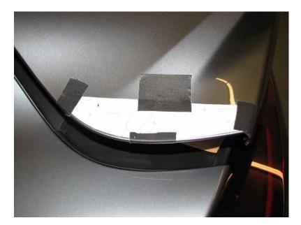
**2.5.** With the template taped in place, place the trunk mount on the trunk with the holes located where the paper template holes are. Ensure that the trunk mount appears to sit on the
