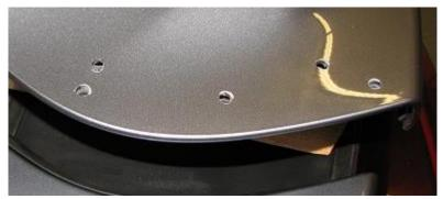
**2.9.** With the all the holes drilled, we can test fit the trunk mount. To do this, install the two studs as shown with a 3mm allen wrench. \*NOTE:\* Not all the studs can be installed and pass through the trunk at the same time, we found these two to work well.
