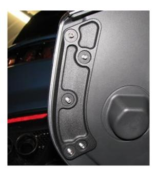
**2.18.** Using stainless washers and the stainless nyloc nuts, tighten the trunk mount and support brace to the trunk to about 6 ft-lbs. The nyloc nuts will resist backing off, so do not go over tighten these.
