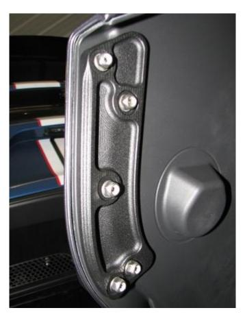
**2.19.** Install the uprights onto the trunk mount by using the M6  $\times$  1.0  $\times$  12mm long button head cap screws and a small washer as shown below.
