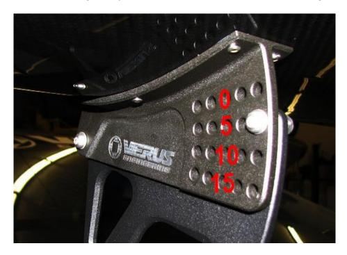
**2.23.** To finish installing the rear wing, we have to install the endplates. We include aluminum washers for M4 flat head cap screws, and O-rings to reduce marring of the carbon fiber.
