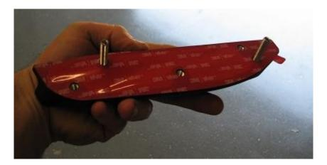
**2.15.** Pull the red side of the double side tape off, and install the trunk mount onto the trunk.
