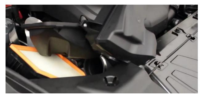
**2.6.** We can now remove the (2) T20 torx bolts holding the resonator on the air box. These are circled in red below.
