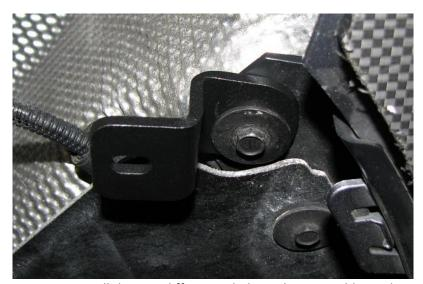
**2.15.** We can now install the rear diffuser. It helps to have an additional set of hands but it is not necessary. On the front (4) locations, we will install the 20mm long BHCS, with a fender washer and a serrated nut on the other side.
