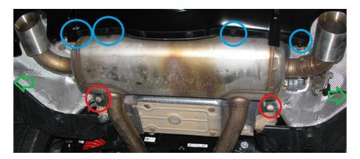
**2.5.** To install the rear mounts, simply remove the OEM 8mm bolt shown below.
