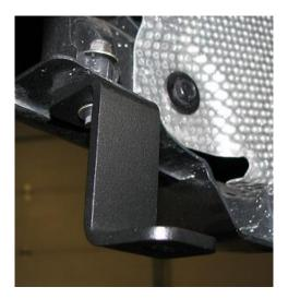
**2.8.** For the inner points that are covered by the heat shield, you will need to cut an opening to access the nyloc nut location.
