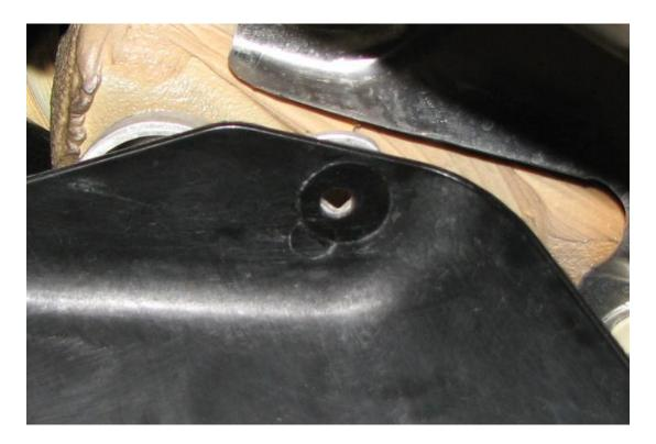
**2.13.** Install the front bracket as shown below. Utilize the M6 x 20mm Long BHCS with a fender washer below, and a serrated nut above the chassis. Note the orientation of the bracket.
