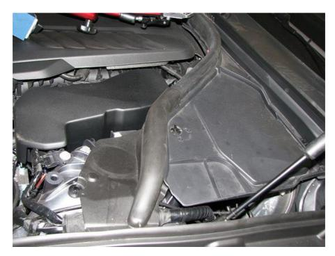
2.4. We will need to remove to plastic covers to gain access to everything necessary for the install. Remove the master cylinder cover by undoing the lock and pulling up and forward.
