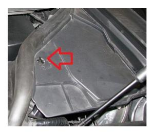
**2.5.** We can now remove the other plastic cover which covers the top of the strut tower area. To do so, remove the two plastic push rivets circled in blue by pulling up on the top section which is shown as an orange arrow.
