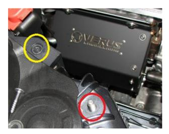
**2.8.** The AOS is now ready to be installed. First we have to assemble the AOS to the bracket with the supplied hardware, as shown below. Tighten the bolts to around 6 ft-lbs.
