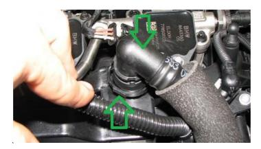
**2.6.** With the hose off the valve cover, we can install the PCV hose adapter as shown below. Simply press it on and it will click into place.
