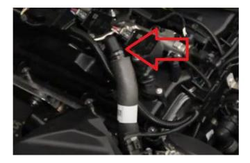
**2.5.** To remove this hose from the valve cover, push the two "ears" on each side of the hose and then pull up. See below.
