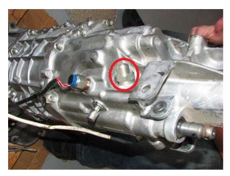
7) Using a 10mm allen hex socket, remove the head straight screw pin, compression spring, and lock ball pin (circled in yellow). Also remove the retaining bolt (circled in blue).
