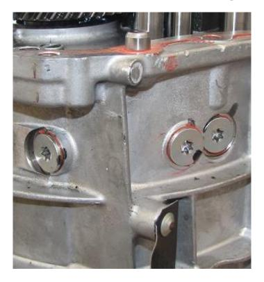
53) Install the final spring pin in 6<sup>th</sup> gear's aluminum shift selector, flush with the outside of the selector.
