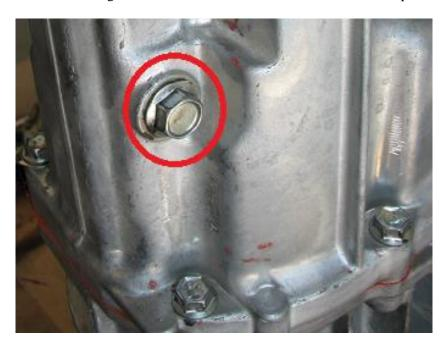
58) Install the 27mm holder with a spring and detent inward in the trans as shown below. Torque to 29 ft-lbs.
