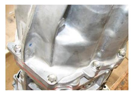
57) Install the bolt with a long tail in the hole shown below circled in red. Torque to 23 ft-lbs.
