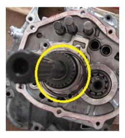
22) Remove the 12mm reverse gear idler bolt and gasket (circled in yellow) and then the other 9 12mm holding the mid-case to the front case/bellhousing (circled in red).
