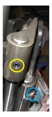
47) Install the below shift shaft. This unit should have a washer and snap ring on it already with a shift head on it as well. If it does not, you will need to install the detent ball on the spring per the service manual (and shown below).
