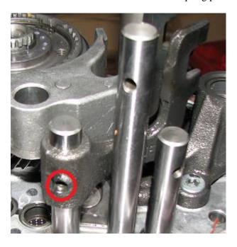
46) Install the remaining two shift heads shown below and drive the spring pins flush (circled in yellow and blue).
