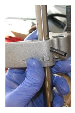
43) Place 6<sup>th</sup> gear, synchro, shift hub, and shift selector on the counter shaft and press the hub on. If you do not possess a press, you can hammer it on slowly but this is not recommended.
