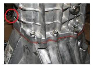
38) Install the other reverse idler bolt with a gasket on. Torque both of these to 21 ft-lbs as well.
