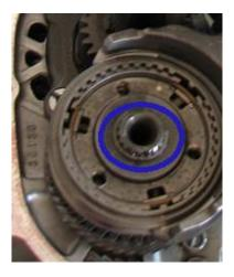
16) Using a steering wheel puller (aka Toyota/Subaru's SST), remove 6<sup>th</sup> gear's synchro hub from the countershaft assembly.
