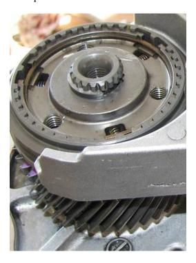
45) Place the shift head shown below on the shaft and drive the spring pin in flush (circled in red).
