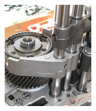
51) While the identification mark is facing as shown (circled in red below), install the final (2) detent balls and springs (circled in blue) in the transmission case. If you look down these holes before installing, you can see a divot for these balls to sink into.
