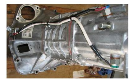
61) Transmission is now ready to be installed back into the engine once you add the shifter and clutch fork/TOB.
