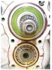
34) Using Toyota's Transmission Sealant (orange), apply sealant to the front cover as shown below. Use grease or generously apply transmission oil on the seal to decrease the chance of ruining the seal.
