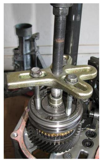
17) Remove  $6^{th}$  gear synchro and  $6^{th}$  gear after synchro hub has been pulled off. Remove the need bearings that  $6^{th}$  gear rides on as well.
