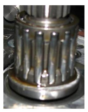
42) Remove the shift selector from 6<sup>th</sup> gear and remove the shaft from the selector by punching out the spring pin as shown below.
