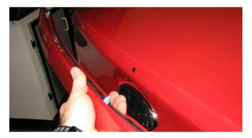
**2.5.** The OE spoiler is now removed and we can clean the area with a 50/50 mix of isopropyl alcohol.
