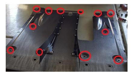
**2.28.** With the diffuser installed on car, we can install the outer strakes with the supplied hardware. On each strake the front (4) bolt holes use the M6 x 1.0 BHCS x 25mm length, M6
