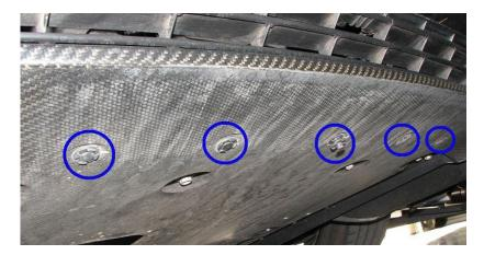
**2.5.** Using the ratchet, 10mm, and 12mm socket, we can remove the diffuser. The 12mm bolts are circled in green below, and the 10mm bolts are circled in yellow. Note, the picture only shows the driver's side of the rear diffuser.
