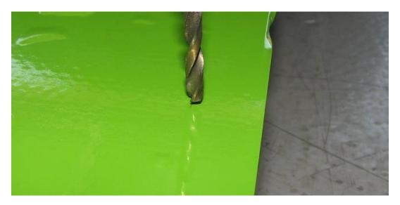
**2.9.** Using a small starter sized drill bit (1/8" will work well), drill through the carbon as straight as possible while staying on the crosshatch. We found high speed and light pressure worked well; let the drill bit cool slightly between drilling.
