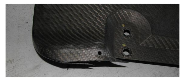
**2.23.** Once you ensure proper fitment of the strake, use some sanding discs to clean up the edges. The rear diffuser will look like below.
