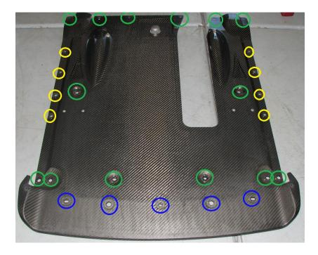
**2.7.** Next, we install the cut template. It will be installed as shown below, match up the exhaust cutout and the two rear holes as closely as possible.
