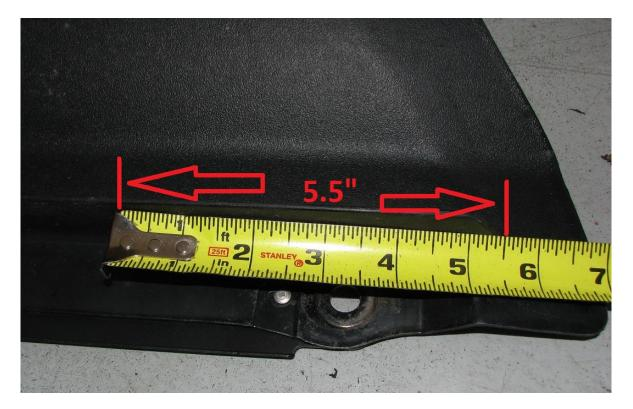
**2.16.** Using the die grinder or a dremel, remove this section and then sand it smooth.
