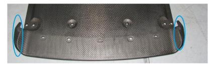
**2.21.** Using the outer strake as a guideline, mark the location that needs slight trimming. This is shown below.
