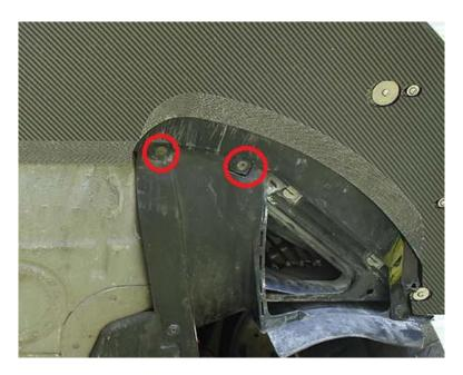
**2.55.** Install the (2) short Torx Head Cap Screws with the 1.00" OD washers in the rear most holes (blue arrow below).
