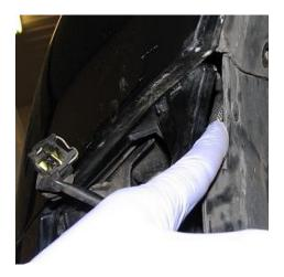
**2.24.** Remove the torx bolt that comes in from the bottom; between the bumper and the fender.
