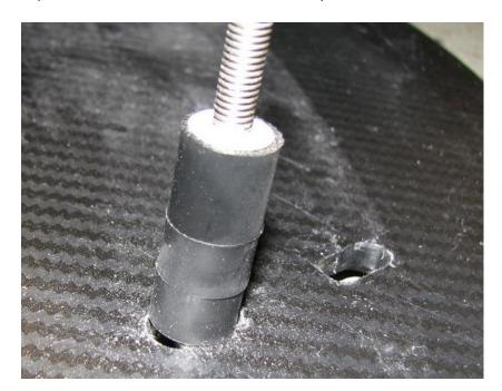
**2.39.** With the (4) bolts installed on the splitter, we can actually begin installing the splitter on the bumper! Do not fully tighten these bolts at this time.
