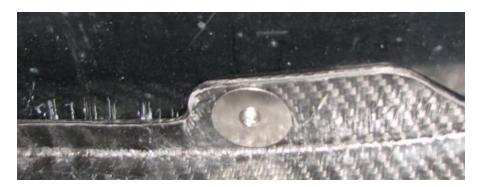
**2.36.** We will now get the front splitter ready for install. \*Note, the bottom side of the splitter has the logo plate on it and is radiused.\*
