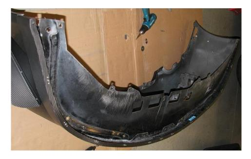
**2.35.** Utilizing (2) of the M6  $\times$  1.0  $\times$  20mm Long BHCS, the large 38mm OD washer, and install these into the air dam to the front bumper locations.
