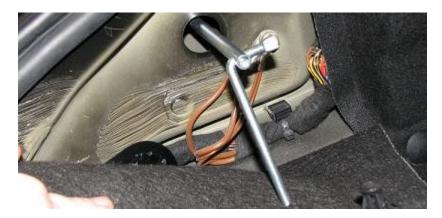
**2.19.** With needle nose pliers, remove the metal pins that hold the top of the bumper to the chassis. There is one per side.
