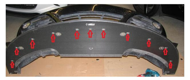
**2.42.** The last two bolts that need installed before final tightening, are the rear most bolts. These utilize a nut on the top and was the reason for cutting a square out of the bumper in step 2.33.
