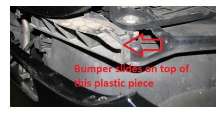
**2.27.** We will need to remove a few harness clips and light clips and then the bumper will be fully free.
