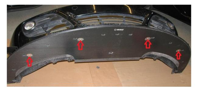
**2.40.** Utilizing the remaining 20mm long BHCS, with the 18mm OD fender washers, to install the splitter to the air dam.
