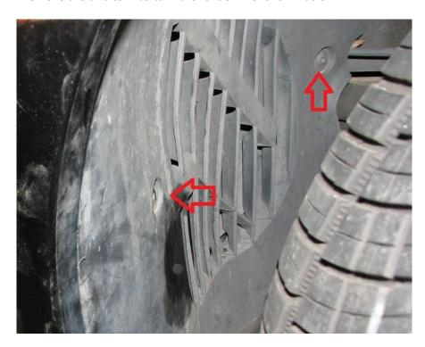
**2.22.** Moving slightly upward in the fender; we remove the following torx bolt.
