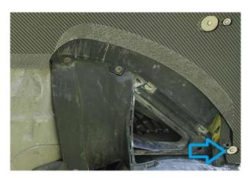
**2.56.** The last bolt to install is the center rear most bolt. Utilize the longer THCS and 1" OD washer. This is circled in green below.
