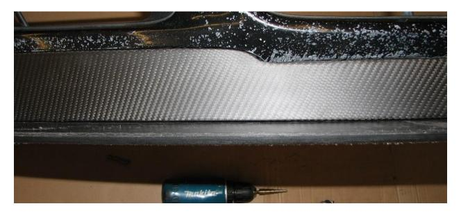
**2.41.** You will need to work the air dam around to get all the holes to line up with the splitter bolts. Install these when you can but ensure you do not cross thread the bolts.
