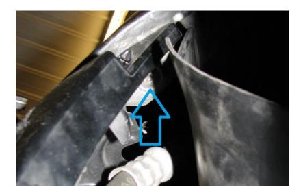
**2.25.** The final seven bolts on the bottom of the bumper needs removed and the bumper can slide forward.
