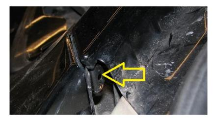
**2.20.** This is what the bumper attaches to via the metal clip when the bumper is removed.
