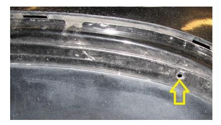
**2.6.** We want to open these holes to 3/8" with a drill and drill bit.
