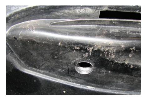
**2.7.** We will now install (4) of the (6) rivet nuts; in the (4) holes we just drilled to 3/8". We will need to grab the install tool and setup the rivet nut for install as shown below.
