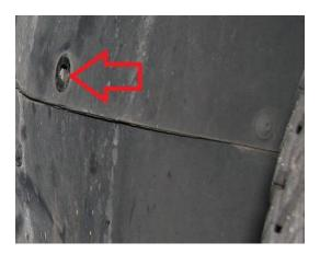
**2.23.** We can now remove the side marker. The side marker is held in place with an A clip in the rear. Pull outward and the side marker should come out.
