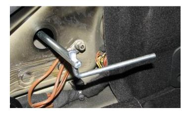
**2.17.** Rotate the handle down and towards the front of the car. This will push the headlight forward.
