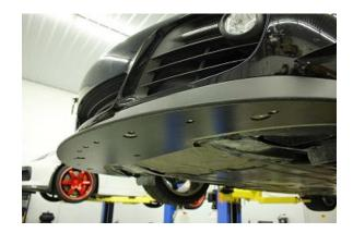
**2.3.** We start by removing the OEM splitter add-ons. These are removed by plastic push pins on the bottom of the bumper. This is then removed by pulling away from the bumper as it clips in on the top side.
