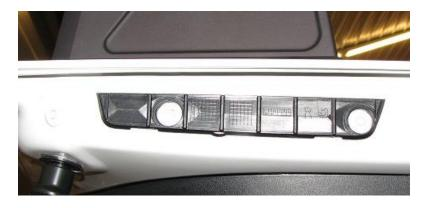
**2.38.** Reinstall the cover by snapping it on in place.
