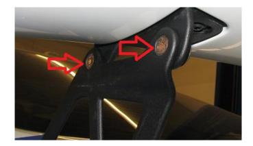
**2.3.** With the wing removed, we can now remove the beauty plate which is double-side taped on. Use painters tape around the beauty plate to protect the paint.
