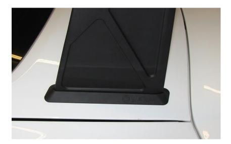
**2.25.** Install the rear wing. It is very helpful to have a second pair of hands for this part as the wing is quite large. Utilize the NAS hardware to install the wing. We recommend starting at 8-10 degrees of AOA.
