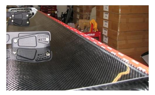
**2.32.** Clean the gurney flap on the surface to be installed on the rear wing.
