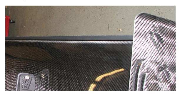
**2.34.** Popping the trunk again, we can install the trunk mounts by simply uninstalling the OEM rubber unit and installing the supplied delrin pieces. These transfer the load of the rear wing to the chassis without deflecting and should be unscrewed until they touch the chassis when fully closed.
