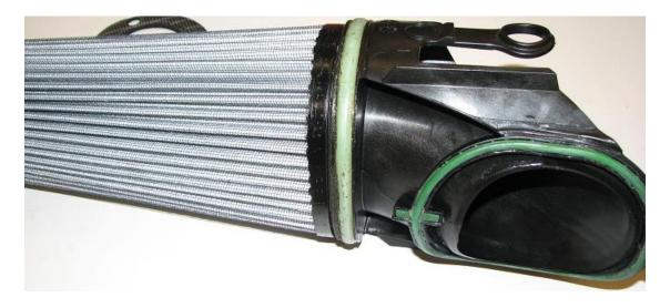
**2.29.** Install and tighten the air filters with the \*supplied\* torx bolts as the thread pitch is slightly different than OEM.
