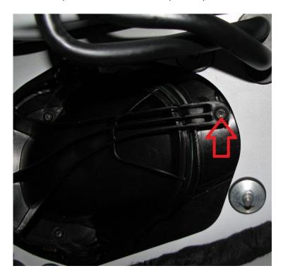
**2.15.** With gloves (Mechanix or something with a bit of cushion), squeeze the two prongs as shown below and pull the air filter from the chassis.
