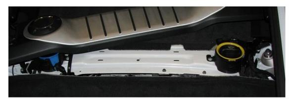
**2.12.** Remove the carpeting so we can access the air filters.
